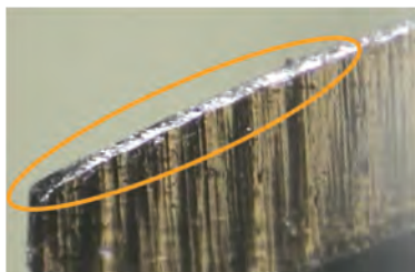
Rounded edge creates cutting issues
