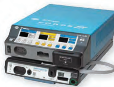
EM3 AEM Monitor connected to the Covidien Force FX electro-surgical generator.
