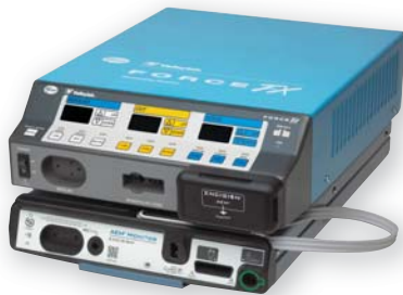
EM3 AEM Monitor connected to the Covidien Force FX electrocautery generator.
